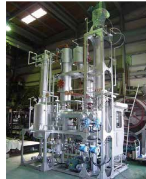
▲ High quality heat de-composition oil equipment
