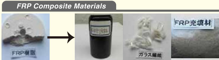
FRP Resin → FRP Dissolved Liquid, Glass Fiber, Filler
